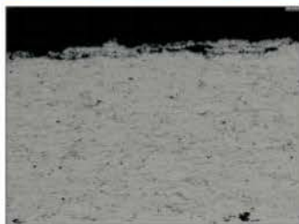
Cross-section metallograph of Cr 3 C 2 -25NiCr coating
