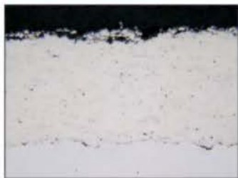
Cross-section metallograph of Cr 3 C 2 -20NiCr coating
