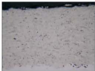
Cross-section metallograph of Cr 3 C 2 -37WC-18NiCoCr coating
