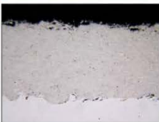
Cross-section metallograph of WC-20Cr 3 C 2 -7Ni coating
