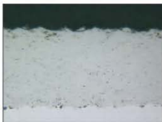
Cross-section metallograph of WC-10Ni coating
