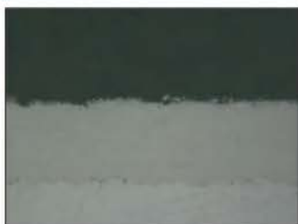
Cross-section metallograph of WC-10Co4Cr coating
