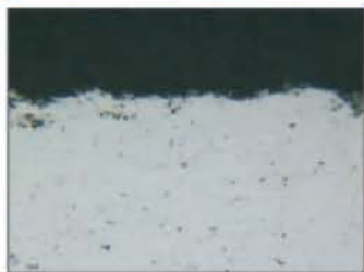
Cross-section metallograph of WC-12Ni coating
