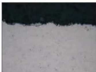
Cross-section metallograph of WC-12Co coating
