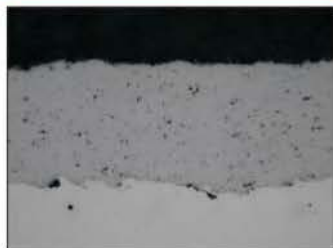
Cross-section metallograph of WC-15NiCr coating
