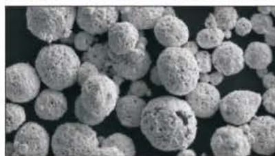
Typical cross-section and surface morphology of WC-10Co4Cr thermal spray powder
