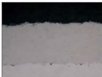
Cross-section metallograph of WC-17Ni coating
