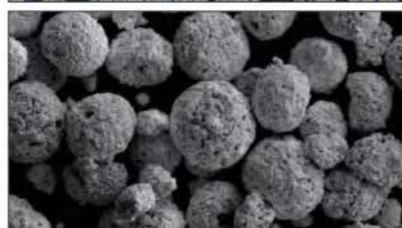
Typical cross-section and surface morphology of WC-12Co thermal spray powder
